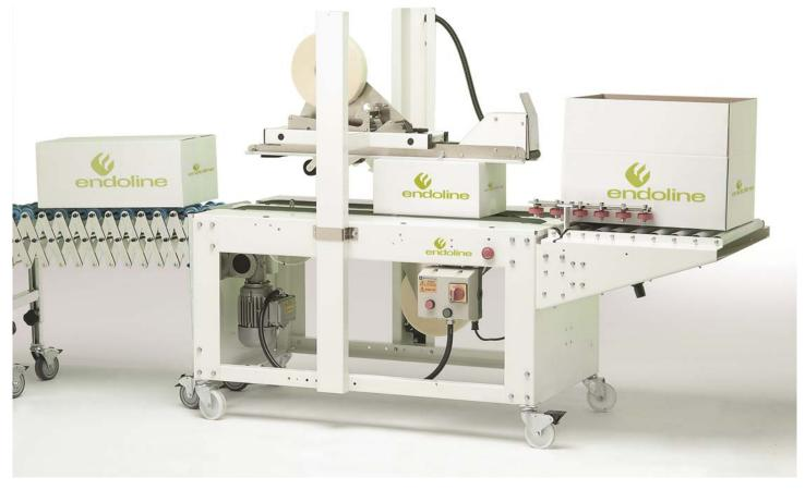
This taper offers the option of a high speed system that can seal random sized cases at speeds of up to 18 per minute, with no manual adjustment for each size of case.
